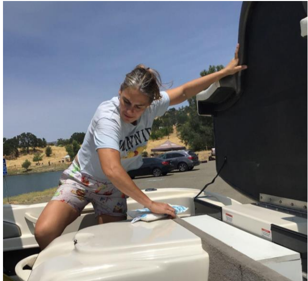
Steele boater installs oil absorbent
