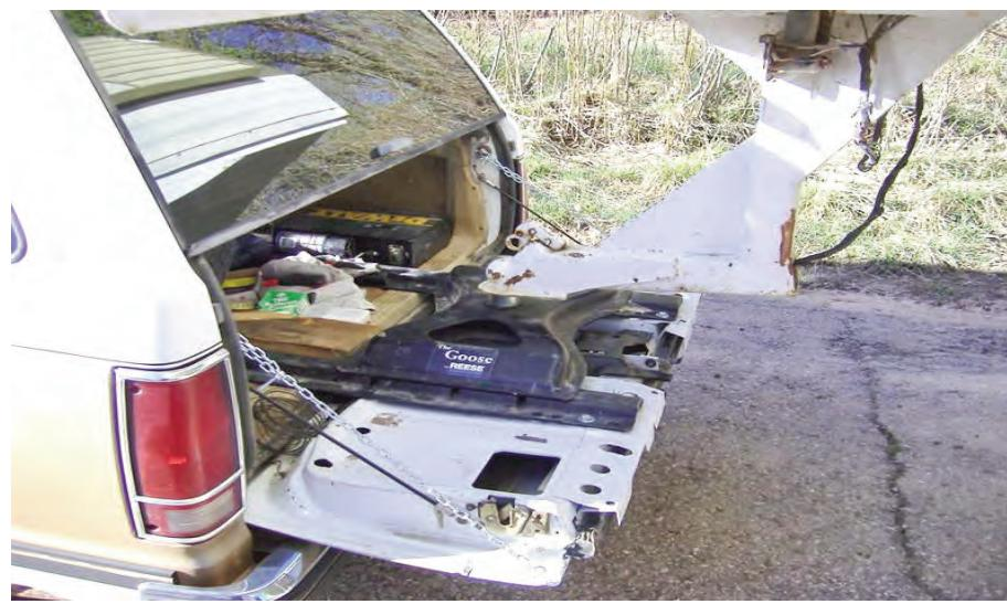
Yep, probably overkill, but you don't want the possibility of having an axer-dent. Spend some time to whittle down that MASSIVE 4x4 to fit precisely into the ball mount receiver. Note the 14"x14" piece of 3/8" plywood on the underside of the ailegate to distribute the load more evenly. B'gosh, it costs a little more but you just CAN'T BE TOO SAFE, Y'ALL!!
